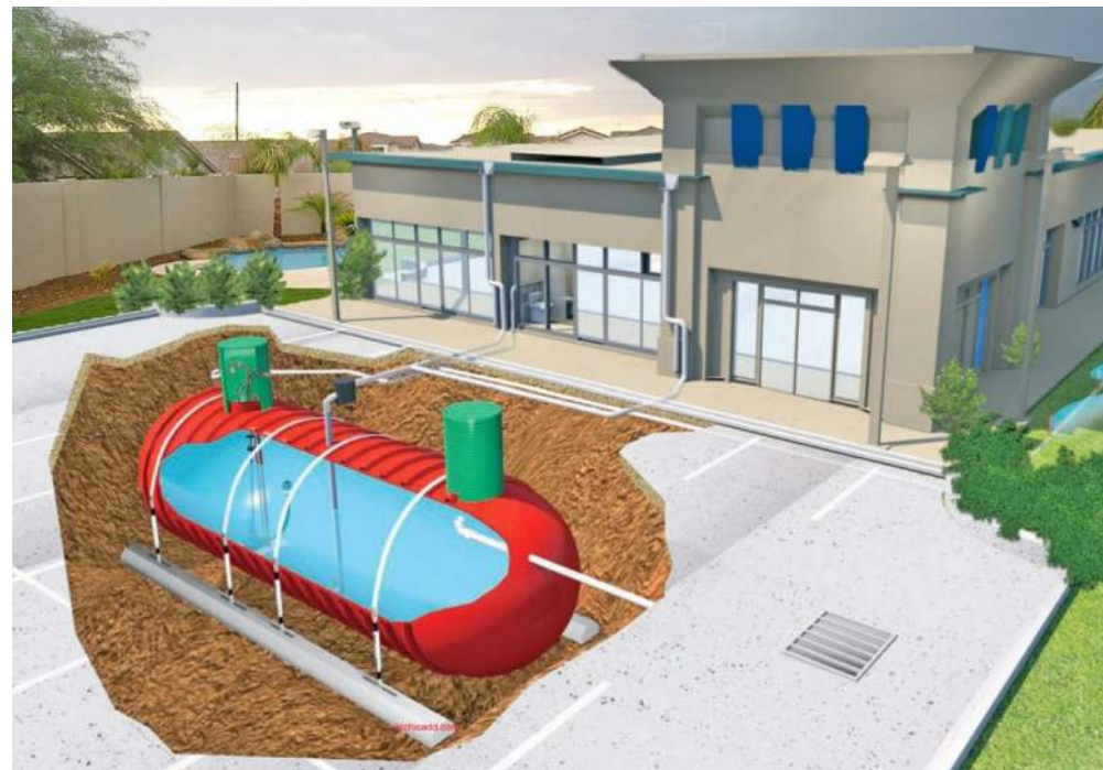
Figure 9.5 – Indicative Rainwater Harvesting Layout
