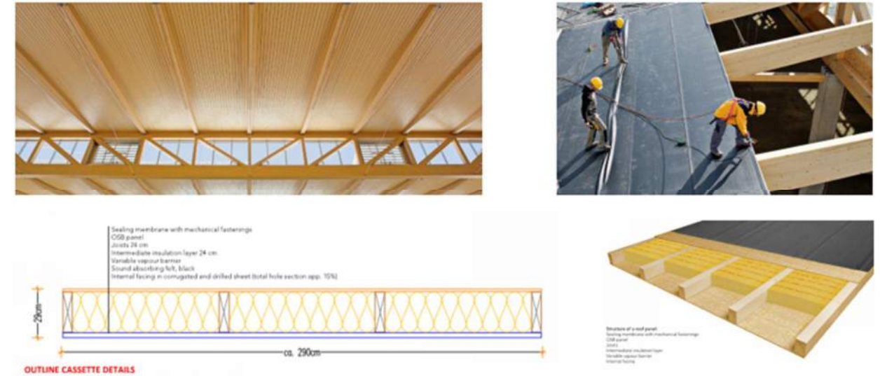
Figure 8.1: Timber Cassette System – Typical Details
